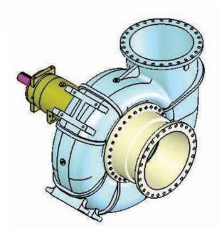
Pumps are made from all iron, horizontal (F) and vertical (VF) configuration with enclosed cast iron impeller, 416 stainless steel shaft sleeve, packing or Cycloseal or double seal, and single casing cast iron wear ring, frame except 4NNTL. All pumps incl. volute clean-out hole & cover.
